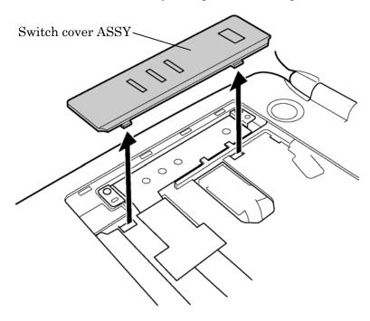
Figure 4-13 Removing the switch cover ASSY
